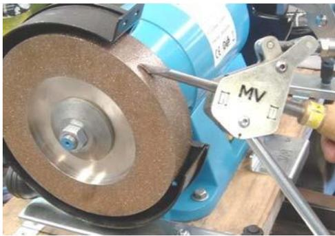
**Flat profile spindle gouges - 33°**
